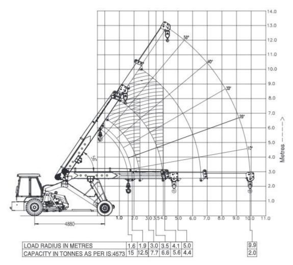
Rated loads are calculated for operation on leveled surface.
