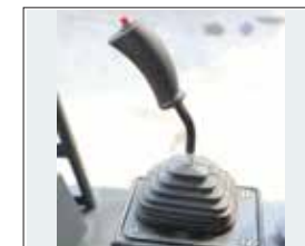
FORWARD REVERSE LEVER WITH VIBRATION CONTROL
